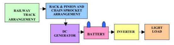
Fig.-1 Block Diagram of Generation of Power Using Railway Track
